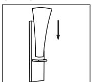
Install proper bulb type and wattage. Slide the glass down.
